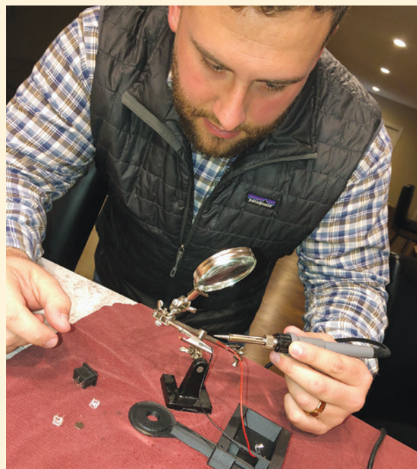
Drew Deathe solders electronic components for a 3D-printed exam scope, which can be attached to a mobile phone for use in assessing trachoma.
